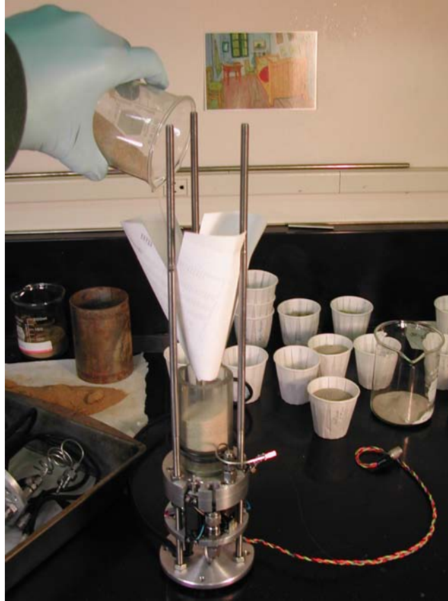
Figure 2.7: The air pluviation technique used to reconstitute the dry samples.
